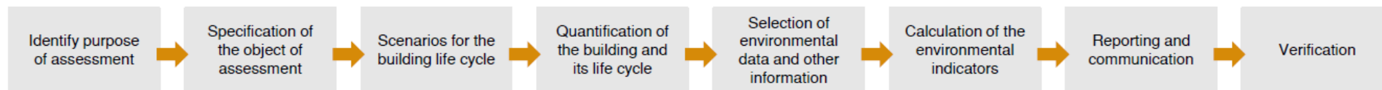
FIGURE 3: Illustration of assessment process (as defined in EN 15978:2011)
